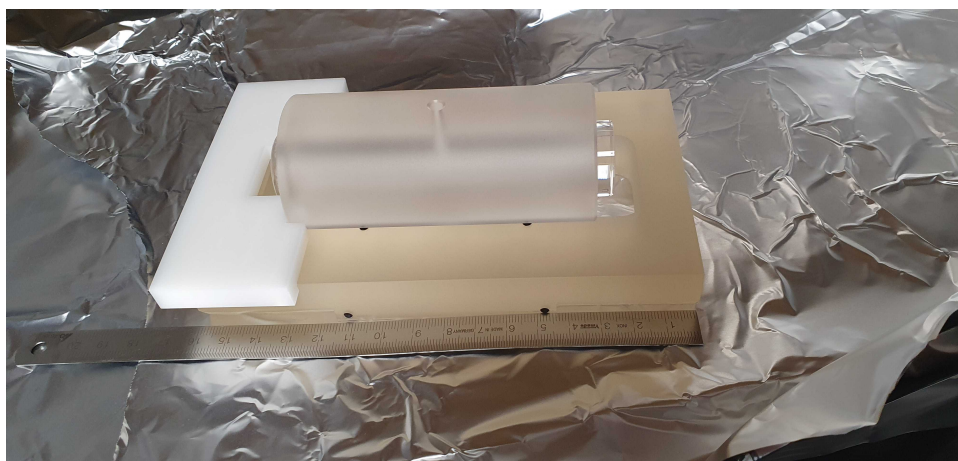
Figure 2.6: Picture of the ULE cavity put onto the square glass mount. The white piece is an alignment tool provided by Stable Laser Systems and is thus removed upon placement of the cavity inside the housing. Four Viton balls on each side of the mount ensure stability from vibrations. The cavity is placed in the center of the mount.
